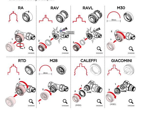
The following adapters are included in the scope of delivery. The other adapters in the overview can be purchased separately. Adapter code number can be found below each adapter illustration.
