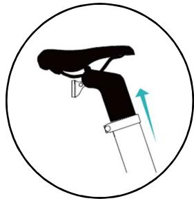
1. Loosen the quick release handle by force.
