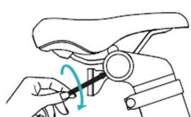
5. Then install the reflector bracket and lock the rear reflector fixing bracket screw clockwise.
