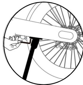
1. First, pre-tighten the parking rack on the frame with two M6\*16 cylindrical head screws (with flat pads).
