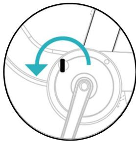
3. Insert the battery key and turn it 180 degrees anti-clockwise to unlock the battery lock.
