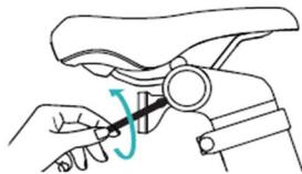
1. Use H3 wrench to loosen the rear reflector fixing bracket screw counterclockwise and remove the reflector.
