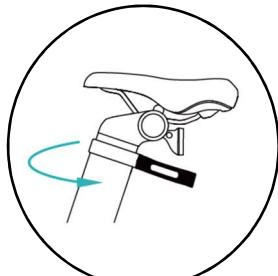
1. Turn off the eBike. Loosen the seat tube clamp by force.
