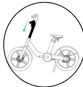
1. Put the handlebar assembly on the frame.
