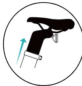
2. Lift the saddle upward and remove the saddle from the seat tube.
