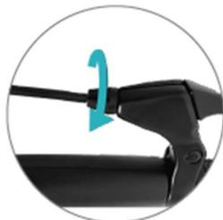
4. Tighten the nut, loosen the disc brake rocker arm, the installation is complete.
