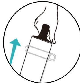
4. Lift the battery upward with force to remove it. Put the battery in the seat tube, then turn the key 180 degrees clockwise to lock the battery and remove the key.
