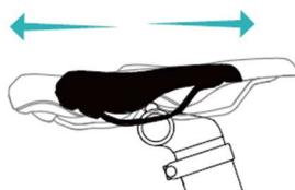
3. The saddle can be moved forward or backward after the saddle tube screw is sufficiently loosened.
