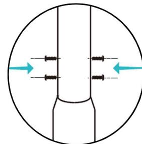
2. Align the screw holes on the handlebar with the screw holes on the vertical tube clevis
