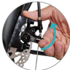
1. Lift the disc brake swing arm upward with force.
