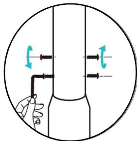
3. Use H4 Allen wrench to pre-tighten four M6\*10 half-round head screws (with bullet pads) on the frame, then tighten each bolt alternately in the order of two lower bolts and two upper bolts until all bolts are tightened.
