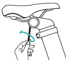
2. Loosen the saddle tube screw counterclockwise with an H6 wrench.
