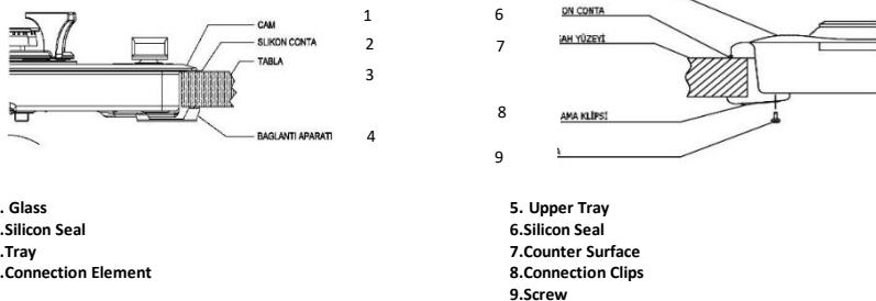
The range is equipped with a seal to prevent the liquids through the cavities into the cabinet. In order to place this seal, adhere the seal as shown in the figures above. Turn the range upside down and remove the protective tape of the rubber seal and adhere it to the range; both ends of the seal should meet each other. Install the mounting sheets as shown in figure 5 by help of screw. And place the range in the opening on the counter.
