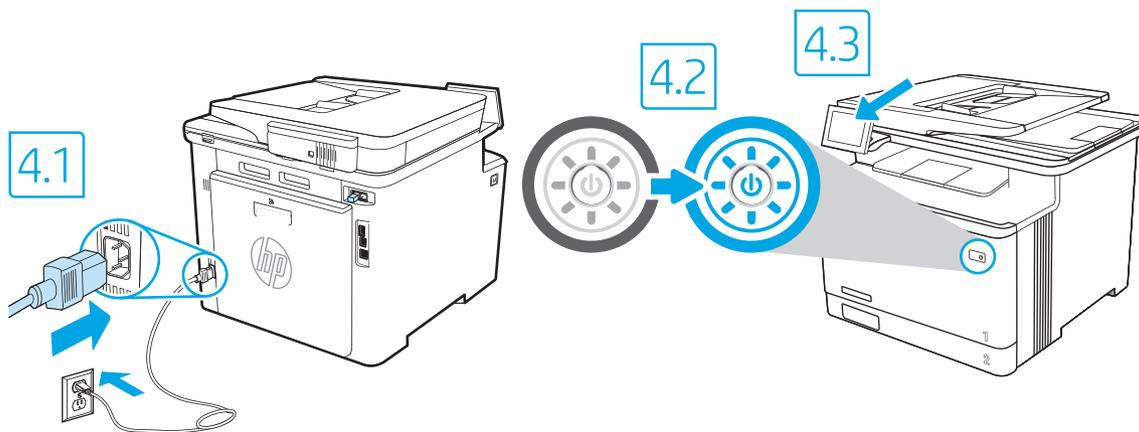
**EN** 4.1 Connect the power cable between the printer and a grounded AC outlet. 4.2 Turn on the printer. 4.3 On the **Initial Setup** screen, set the language, the location, the date/time format, and other features.
