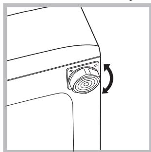
Levelling the machine correctly will provide it with stability, help to avoid vibrations and excessive noise and prevent it from shifting while it is operating. If it is placed on carpet or a rug, adjust the feet in such a way as to allow a sufficient ventilation space underneath the washing machine.
