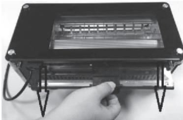
To reinsert the glass panel, lay the toaster on its back, then hold the panel by the latch and carefully slide it back into the grooves at the side until it clicks securely into place.
