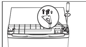
4. Unscrew bottom hinge of freezer door. Then remove the door and place it on a soft pad to avoid scratch.
