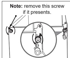
4. Unscrew and remove the bottom hinge pin, turn the bracket over and replace it.
