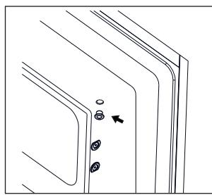
7. Rotate freezer door and place hinge side at left side.
