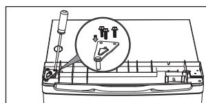
13. Put the top cover and fix it with 2 screws on the back.
