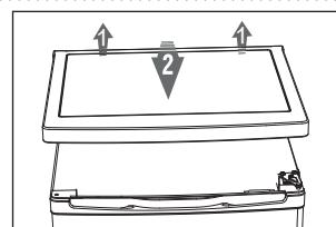
3. Unscrew top hinge and then remove door and place it on a soft pad to avoid scratch.
