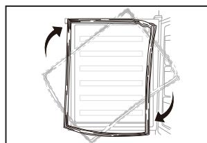
12. Place the door back on. Ensure the door is aligned horizontally and vertically, so that the seals are closed on all sides before finally tightening the top hinge.
