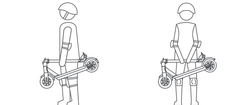
Fold and hold the handlebar rod with one or both hands.
