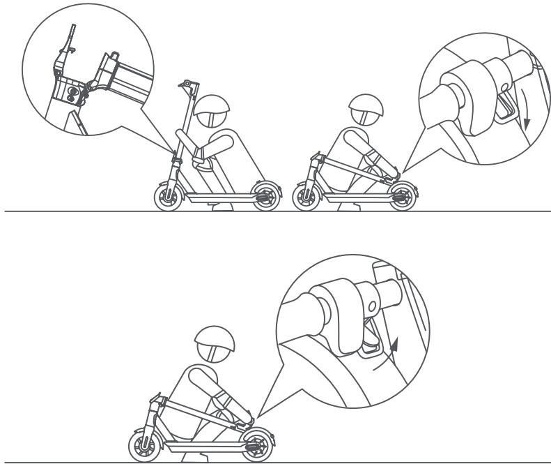
Make sure that the electric scooter has been switched off. Hold the handlebar rod with your hand, then pull the lever and align the handlebar hook with the hook located on the footboard.
