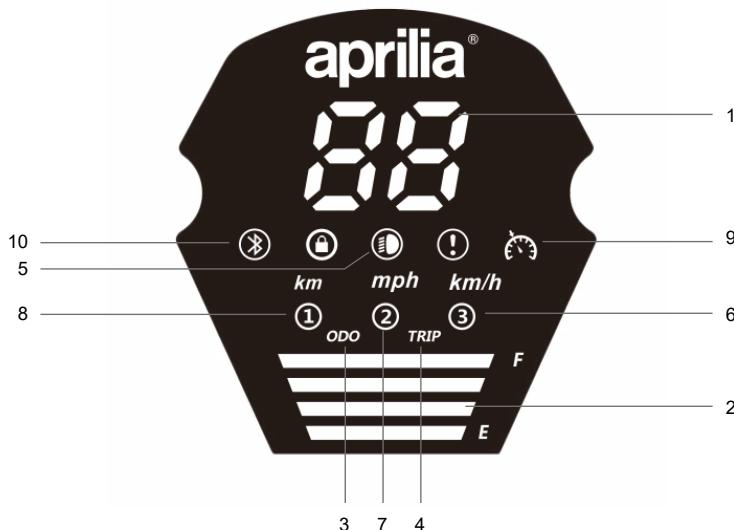
1. Speedometer: Displays the current speed of the scooter.
