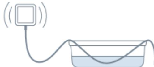
Submerge the sensing cable in water during alarm test. This will result in a gentle test alarm. After the successful test, Eve Water Guard will return to normal mode.
